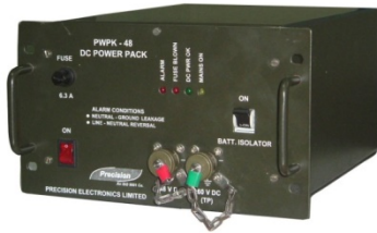
Stand Alone Power Pack: MIL-grade SMPS based Rectifier with Power conditioning and Float/ Boost Charging
