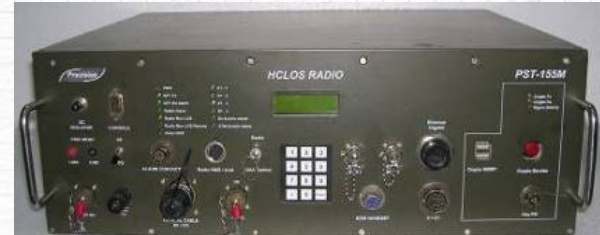
PST-155M: Secure HCLOS Radio for Tactical and Strategic Networks. Supports up to 155 Mbps
