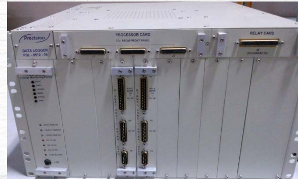
Data Logger: used by the Railways to log, archive, analyze and replay all analog and digital sensor inputs at a train platform
